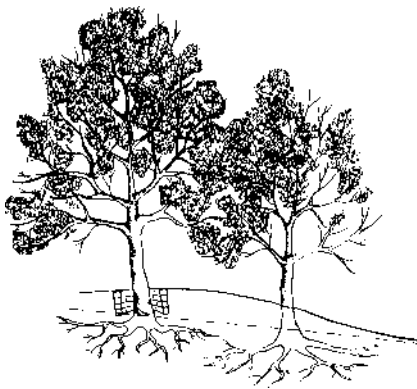
Fill injury from raised grade
